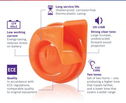
The Economic Commission of Europe (ECE) specifies that audible warning devices for passenger vehicles (such as horns) are required to produce a sound pressure level (SPL) within 105 - 118dB(A). The Bosch Evolution fanfare horns fulfil this requirement while using less electricity.
