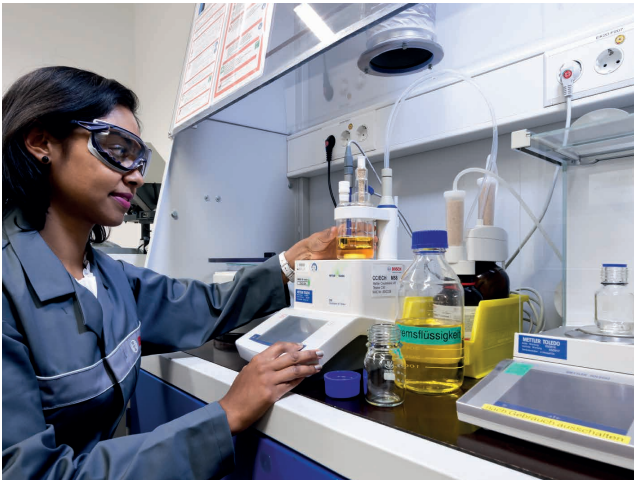
Bosch ENV6 test results at the laboratory: At the Bosch development center, the brake fluid is subject to chemical tests.
