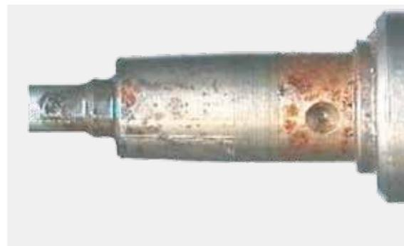
Corrosion at the injector
