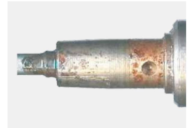
Corrosion at the injector
