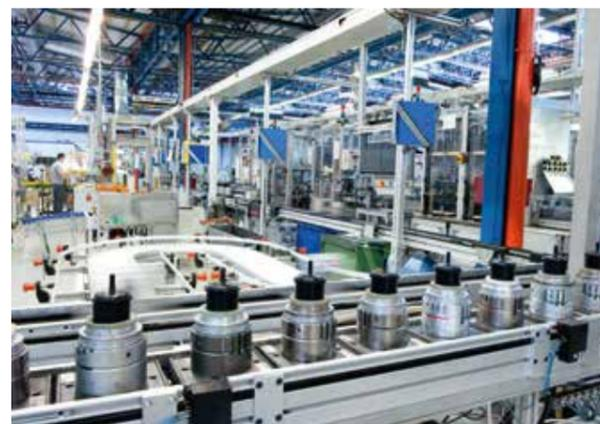
Gasoline-filter assembly line
