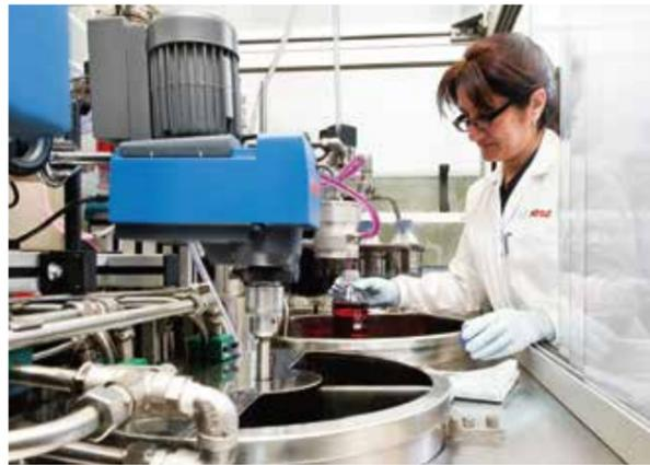
Optical particle counting when testing filter efficiency
