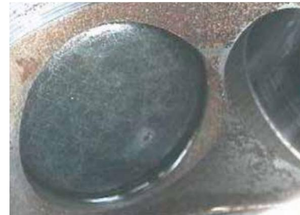
Corrosion at the high-pressure pump housing
