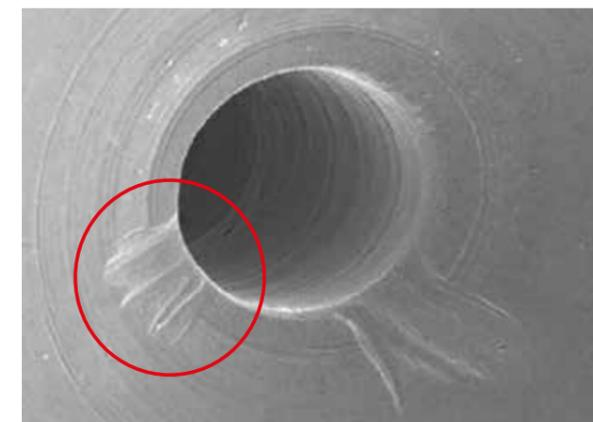
Material abrasion on the injector
