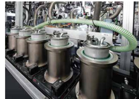
Air-helium leakproofness test
