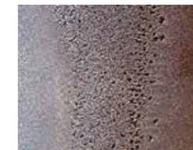
Insufficient coolant filtration can result in pitting. The result: damage to the cylinder due to corrosion.
