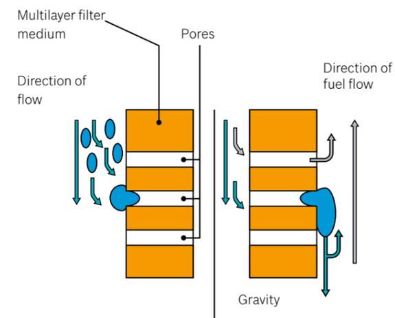
Water separation on the clean side of the filter, small water droplets combine into larger water drops as they flow through the pores (= coalescence effect). These larger drops then drop down.
