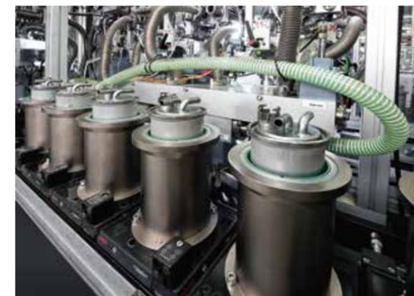
Air-helium leakproofness test
