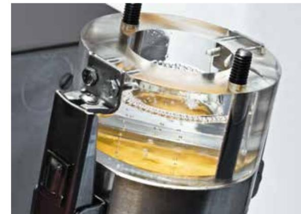
Measurement of the maximum pore size
