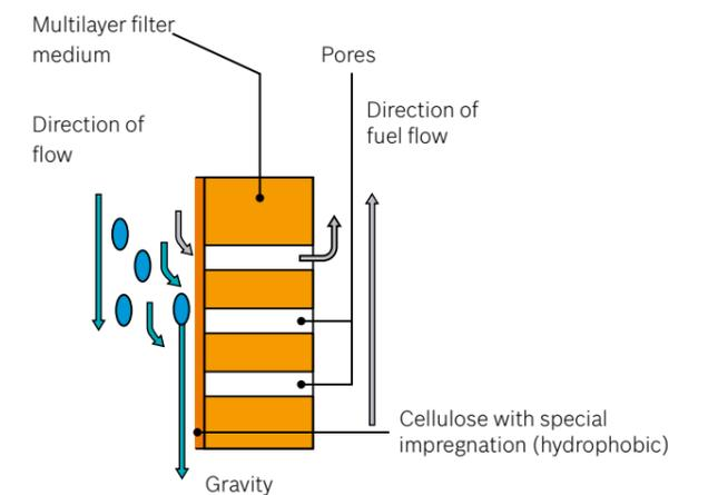
Water separation on the dirty side of the filter thanks to a filter medium coated with a water-repellent (hydrophobic) special resin.
