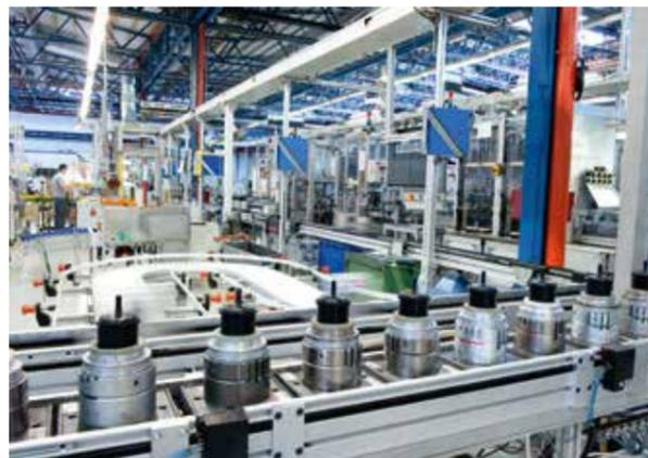
Gasoline-filter assembly line
