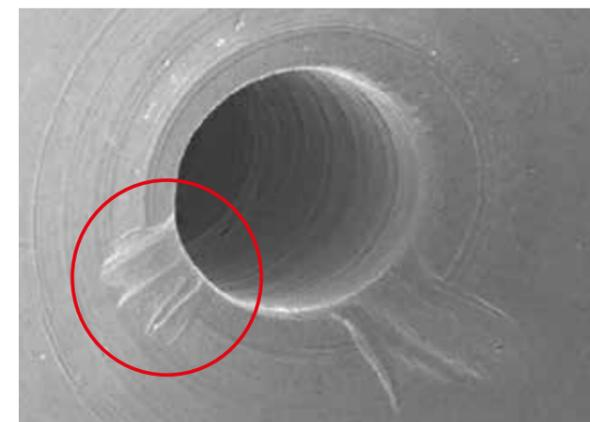
Material abrasion on the injector
