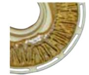
Corrosion caused by spray water
