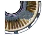
Damaged, porous seal
