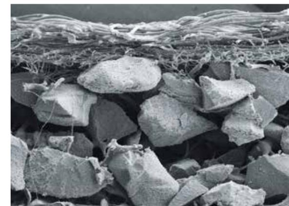
Activated carbon observed under the microscope
